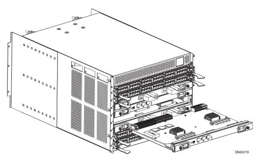
Figure 35. Removing the control processor (CP8) blade
